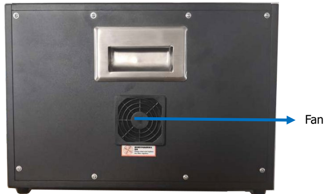
Figure 7-3 Side panel of the control box
