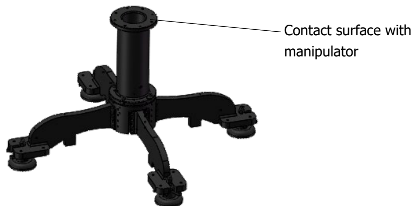
Figure 6-3 Diagram of manipulator base structure
