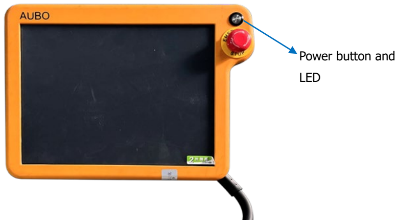
Figure 9-1 Teach pendant and the power button
