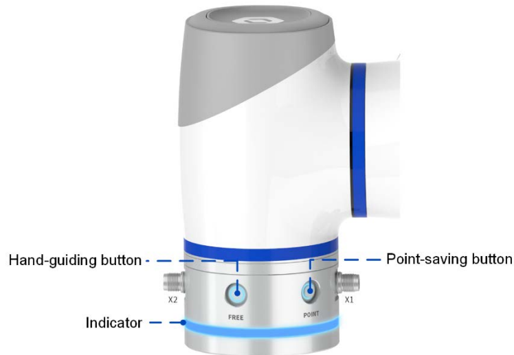
Figure 2.8 Tool flange buttons and indicator (CR20A/CR20AF)
