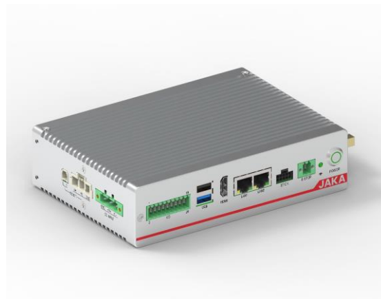
Figure 3-2 The practicality picture of JAKA MiniCobo and MiniCab controllers
